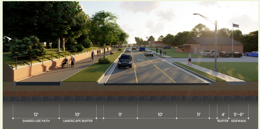
Proposed typical section just south of N. Green Street intersection, facing south
